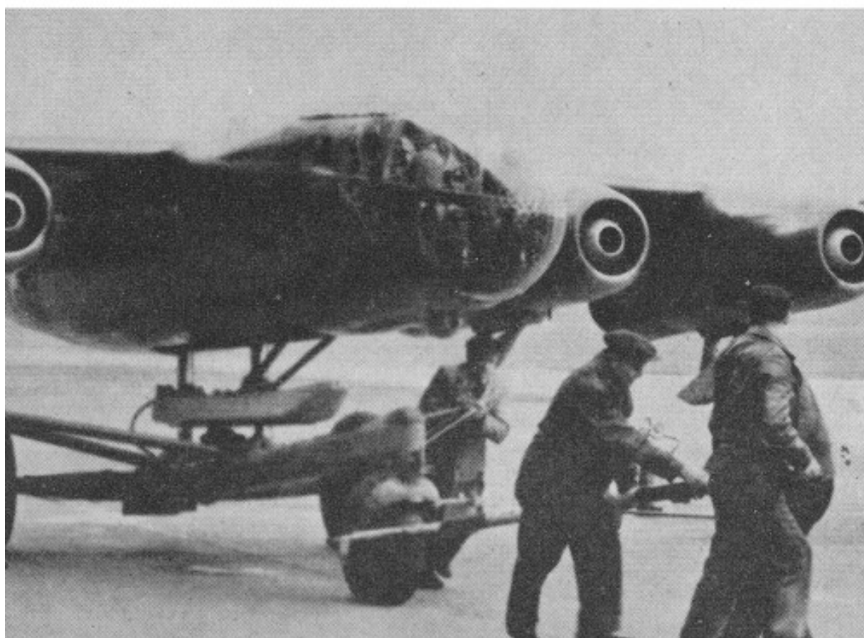
A four-jet airplane with a speed of 670 mph, the Arado AR-234 was designated as a fighter! It carried a two-ton bomb in its concave underside. ( Air Force Photo )
